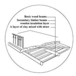
II. 5. Traditional constructive isometric section (scheme credit H. Abass)
