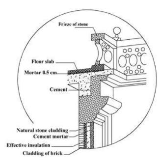
Il. 6. Section through the wall, showing the layers of building materials in French Mandate period (scheme credit H. Abass)
